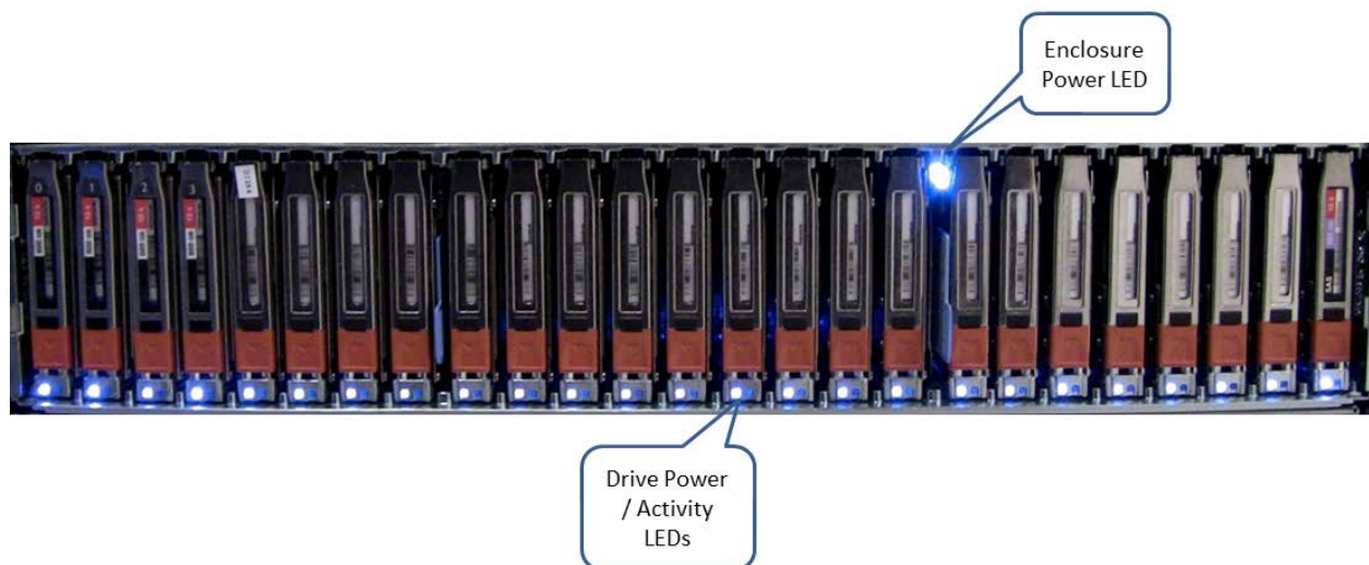
Figure 22. Front of a 25-drive DPE with 2.5" drives
