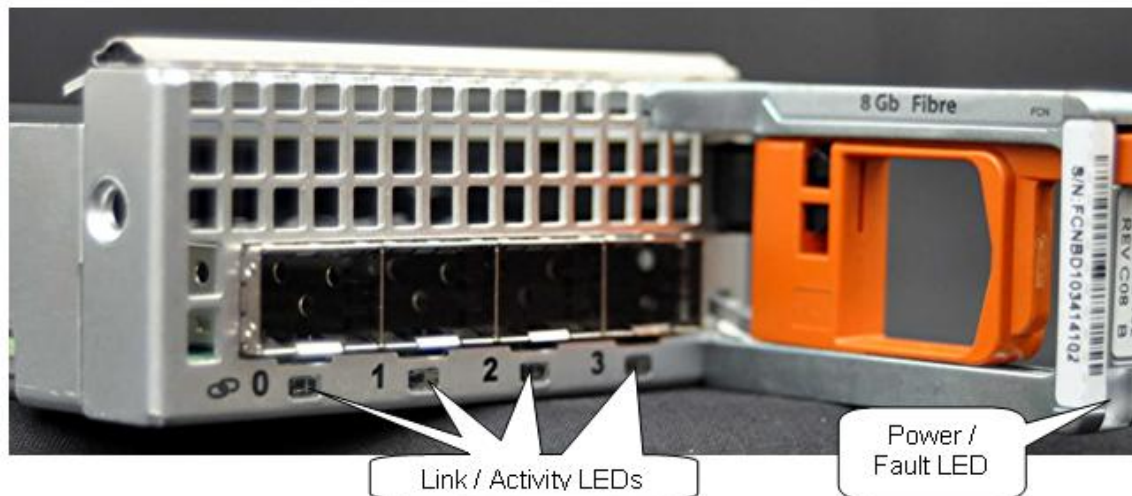
Figure 32. The quad-port 8 Gb/s FC optical I/O module
