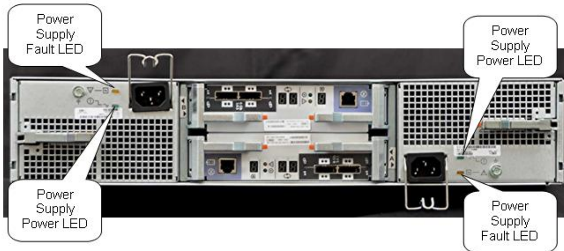
Figure 6. Back of the 25-drive DAE housing 2.5" SAS drives
