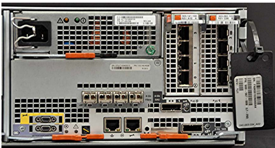
Figure 19. A close-up of the back of the DPE-based storage processor
