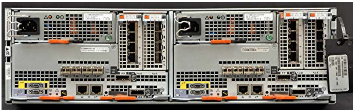
Figure 18. Back view of the DPE with SP A (on the right) and SP B (on the left)
